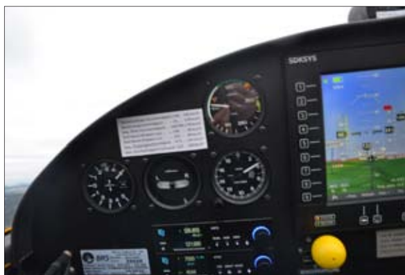
The instrument panel: analog instruments as backup, two TQ radios, and a BRS rescue system; the yellow button operates the tow release.
