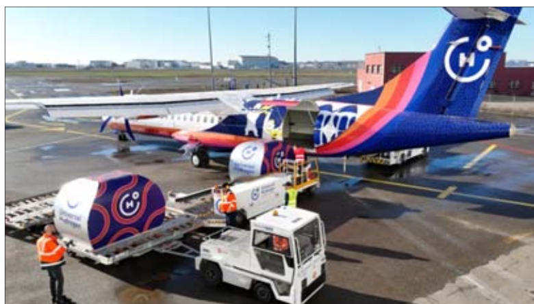
The modular hydrogen distribution system at the airport envisioned by Universal Hydrogen
