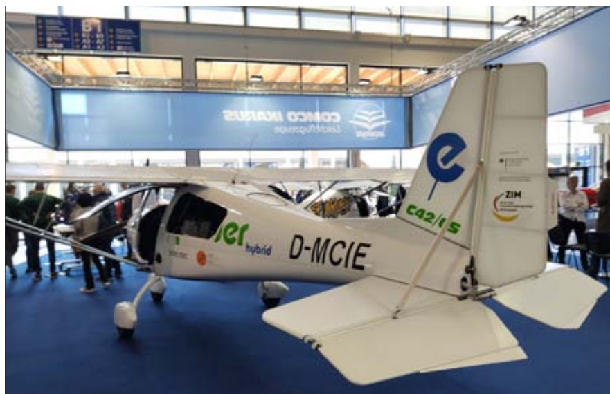
Ikarus C42 with fuel cell and electric motor
