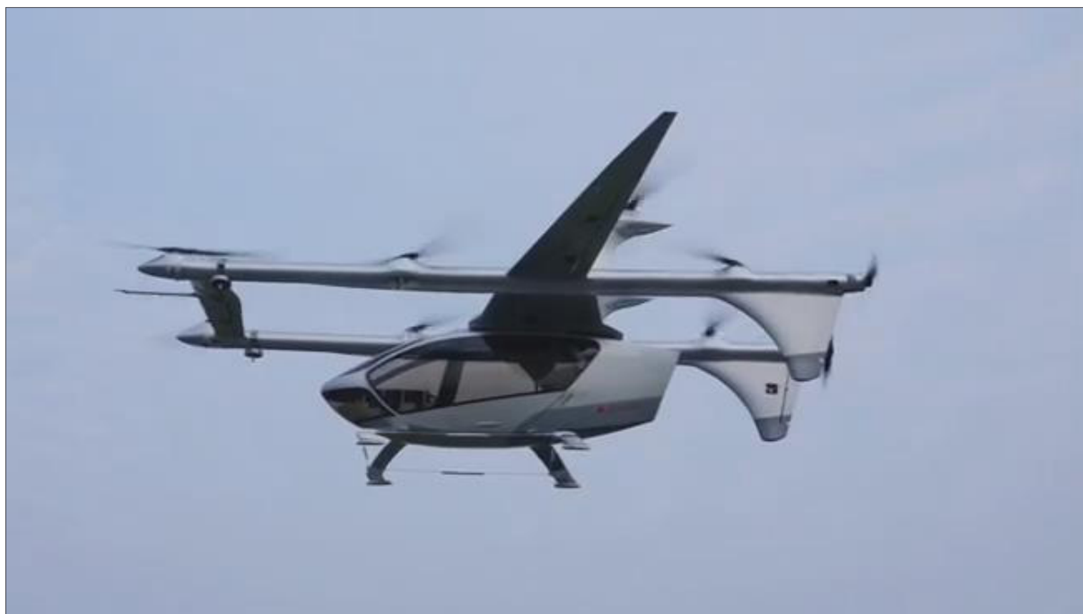
The passenger-carrying model of Prosperity I. There're two propellers at the end of the beam
