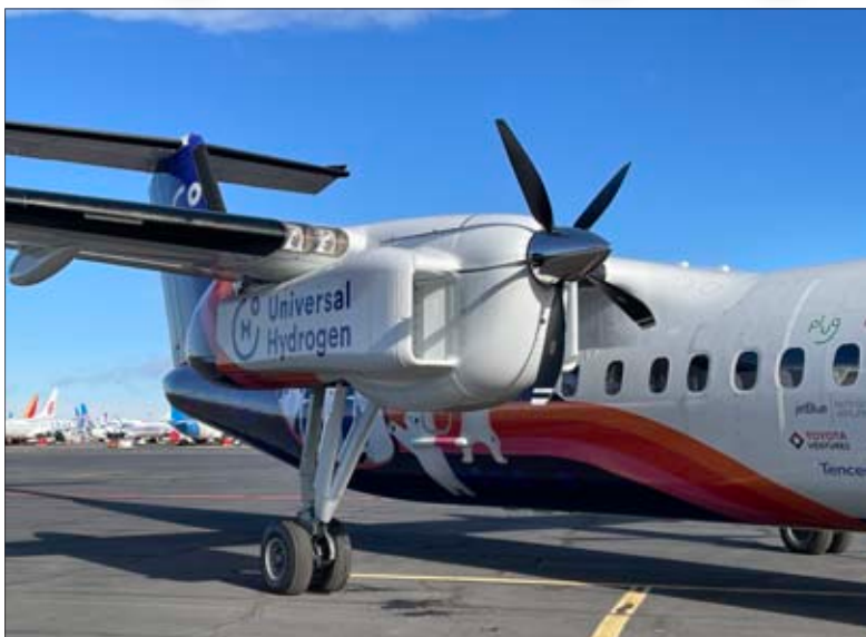
One turbine engine on the Dash-8 demonstrator of Universal Hydrogen was replaced with a 750kw electric motor powered by hydrogen fuel cell
