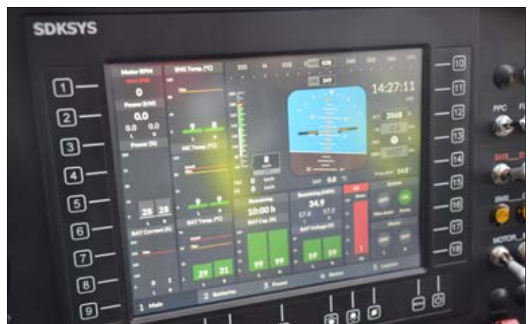
The display is a high-performance computer with military security standards: it runs both the nav, the engine monitoring, and the DAP, which monitors the aircraft, records the data, and transmits it live.
